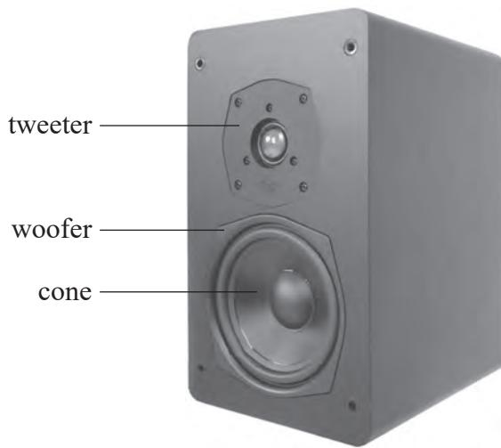
A signal applied to a coil attached to the centre of each cone causes the cone to vibrate and set the air into vibration.
